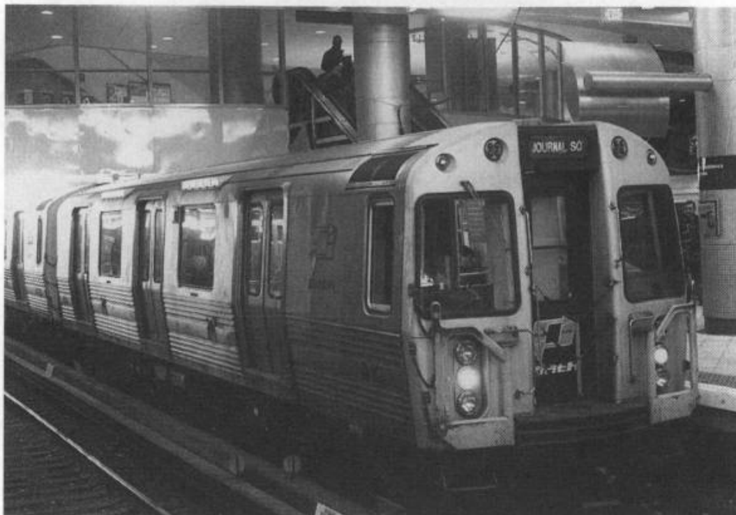
A train of PA-4 units is about to depart Journal Square for 33rd Street in midtown Manhattan. A major difference between PA-4 equipment and earlier PA cars is the inclusion of three sets of doors along each side of the newer equipment.
